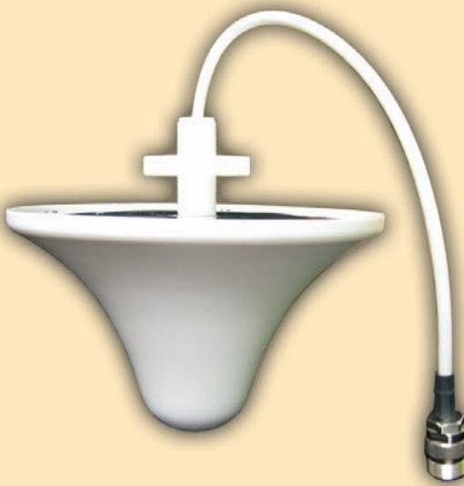
Digital Antenna's multi-band ceiling mount antenna is designed to be mounted indoors on a suspended ceiling having either flush or recess mounted ceiling tiles. This 3 dB gain ceiling mount antenna adds an attractive low profile appearance to a repeater installation. Ideal for use with all Digital Antenna PowerMax™ 4KSBR-50U and 4KMR-30U repeaters. Also for use with 2.5 GHz WiFi systems.
